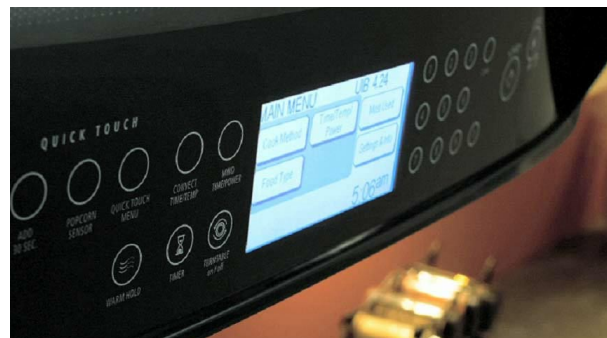
Fig. 7 - Whirlpool Velos™ oven with a single-chip QMatrix part driving 21 conventional touch keys plus 10 clear ITO-film buttons to create an LCD touchscreen. This design uses a 1-layer CEM-1 PCB for very low cost.
