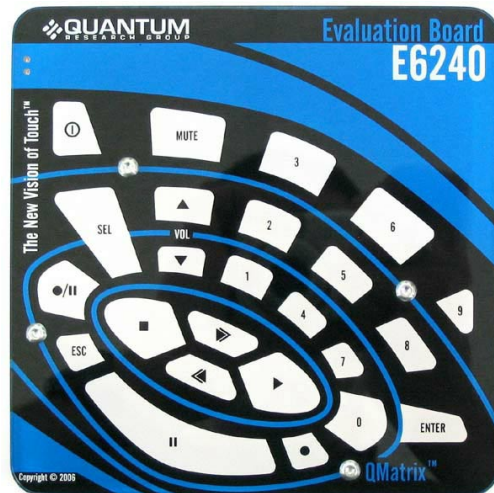
Fig. 8 - Quantum sells QMatrix demo boards such as this E6240 unit, to allow user evaluation of the technology. This board demonstrates the ability of QT6 family devices to sense a wide variety of key sizes and layouts. These boards also work with QmBtn PC software for complete visualization of the signals in real time.
