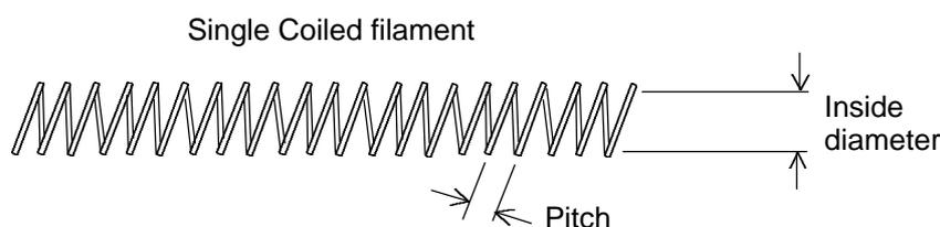
The closer the spacing of the coils, (known as the pitch), then the hotter the filament can operate.
