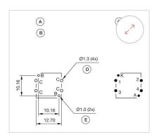
A = Switching element with illumination B = Single LED
