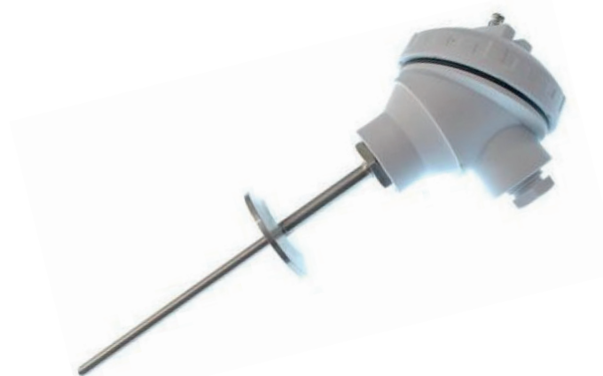
Platinum Resistance Pt100 Hygienic Thermometer, 1.5" Tri-Clamp fitting
