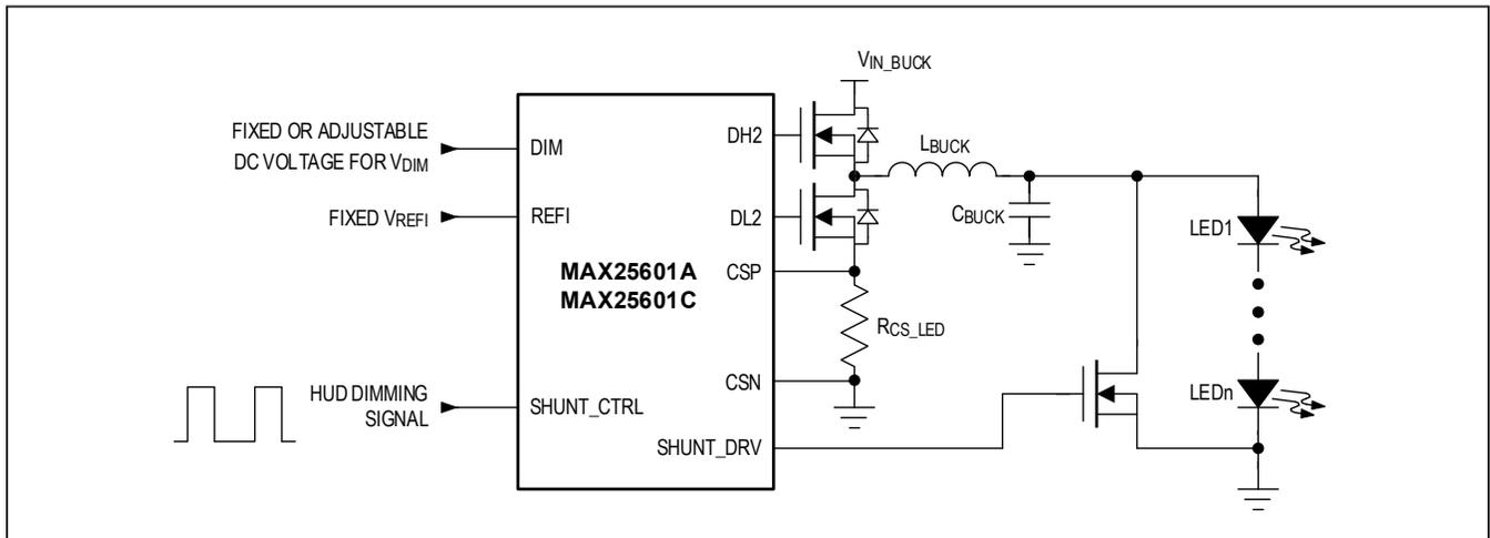
Figure 7. Shunt Dimming
