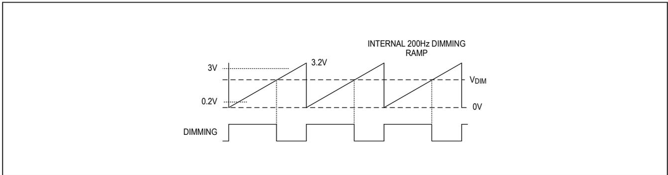
Figure 6. Analog-to-PWM Dimming
