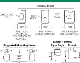
"Push-On" Type Retaining Nut for Quick Mount Fuseholder
