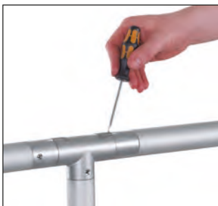
Release stopper with a screwdriver
