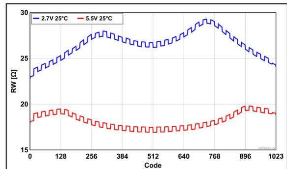
**FIGURE 2-16:** Wiper Resistance ( $R_W$ ) in Rheostat Mode vs. Wiper Position (Code), across  $V_{DD}$  and Temperatures.
