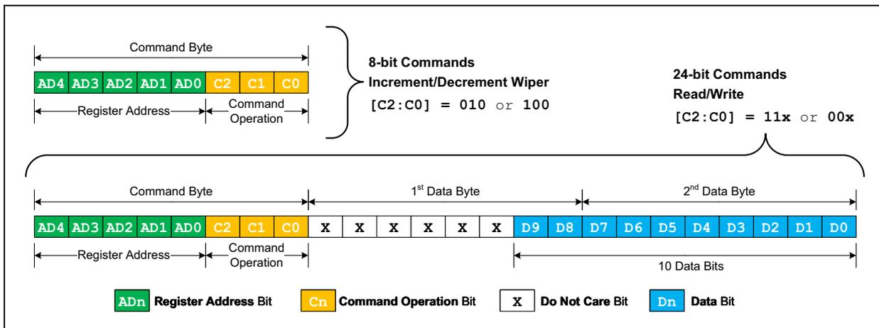
FIGURE 7-6: General SPI 8-Bit and 24-Bit Command Formats.
