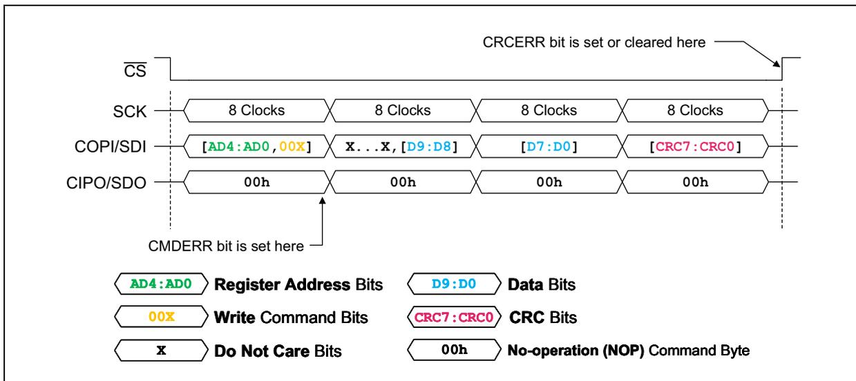
FIGURE 7-17: SPI Write Command Sequence with CRC Enabled.
