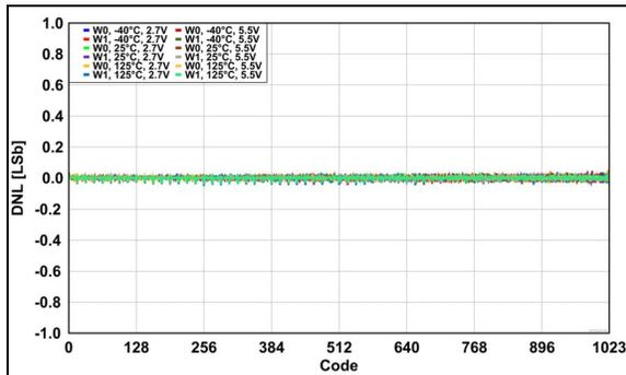
**FIGURE 2-23:** Potentiometer Differential Nonlinearity (P-DNL) Error vs. Wiper Position (Code), across  $V_{DD}$  and Temperatures.
