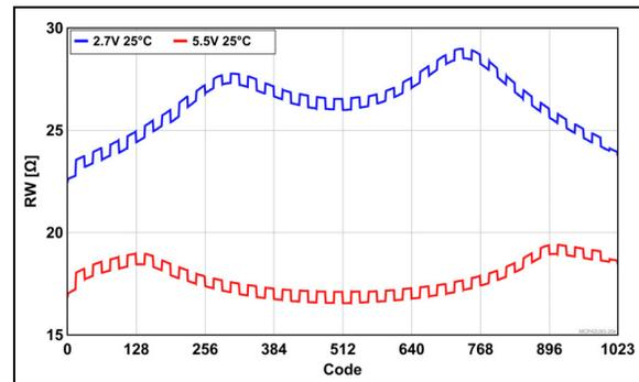
**FIGURE 2-21:** Wiper Resistance ( $R_W$ ) in Rheostat Mode vs. Wiper Position (Code), across  $V_{DD}$  and Temperatures.
