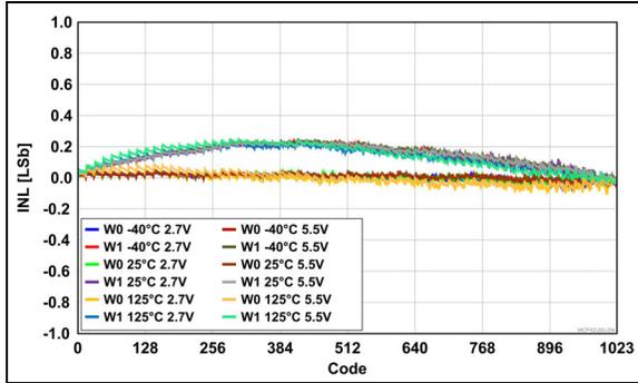
**FIGURE 2-17:** Potentiometer Integral Nonlinearity (P-INL) Error vs. Wiper Position (Code), across  $V_{DD}$  and Temperatures.
