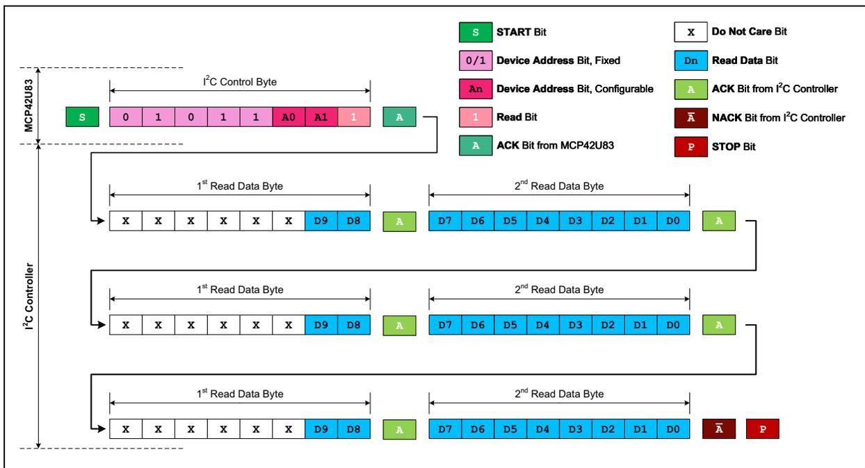
**FIGURE 6-10:** I<sup>2</sup>C Continuous Read of Last Memory Address Command Sequence.
