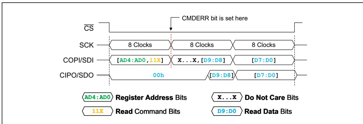
FIGURE 7-8: SPI Read Command – SDI and SDO States.
