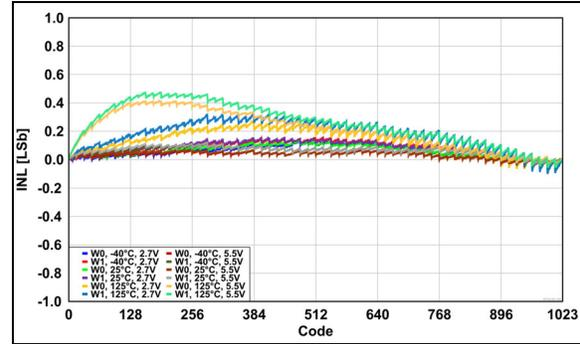
**FIGURE 2-29:** Rheostat Integral Nonlinearity (R-INL) Error vs. Wiper Position (Code), across  $V_{DD}$  and Temperatures.
