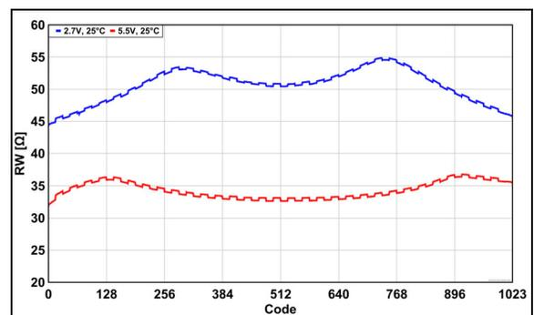
**FIGURE 2-26:** Wiper Resistance ( $R_W$ ) in Rheostat Mode vs. Wiper Position (Code), across  $V_{DD}$  and Temperatures.
