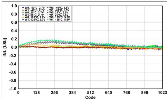
**FIGURE 2-22:** Potentiometer Integral Nonlinearity (P-INL) Error vs. Wiper Position (Code), across  $V_{DD}$  and Temperatures.
