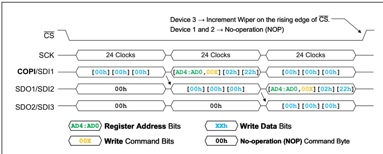
FIGURE 7-15: SPI Daisy-Chain Addressable 24-Bit Write Commands Example.
