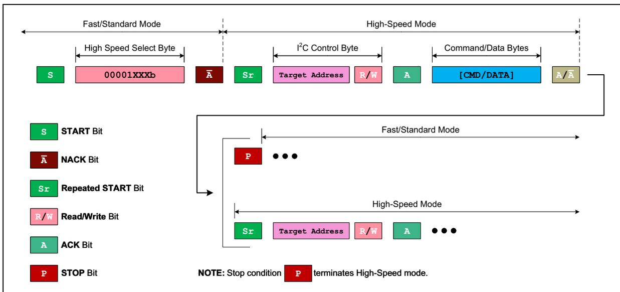
FIGURE 6-3: I<sup>2</sup>C High-Speed (HS) Mode Communication Sequence.
