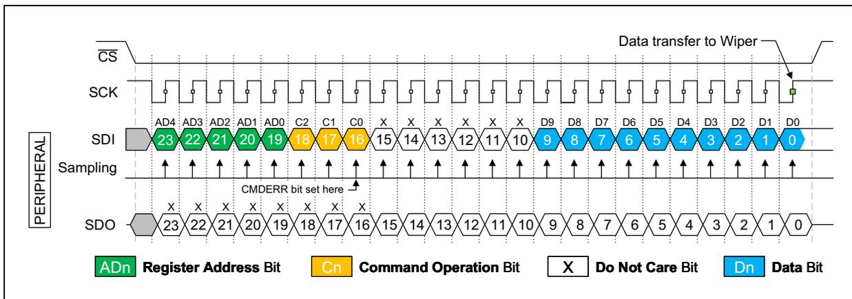
FIGURE 7-3: 24-Bit Commands (Write, Read) – SPI Mode (1,1) Waveform.
