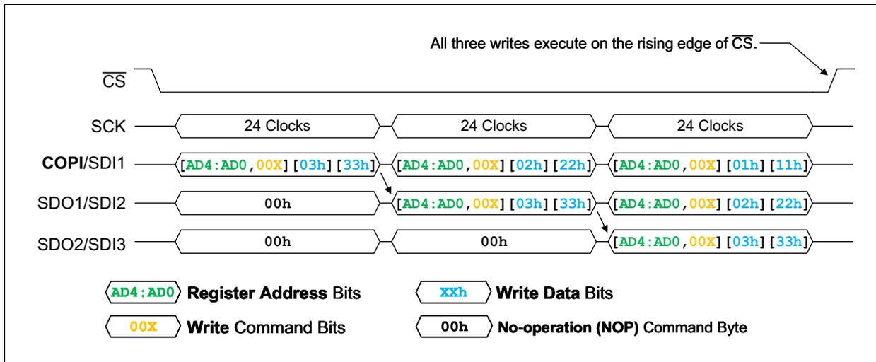
**FIGURE 7-13:** SPI Daisy-Chain 24-Bit Write Commands Example.
