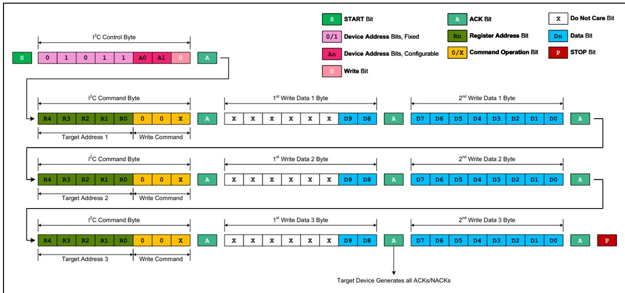
**FIGURE 6-7:** I<sup>2</sup>C Continuous Write Command Sequence Example.
