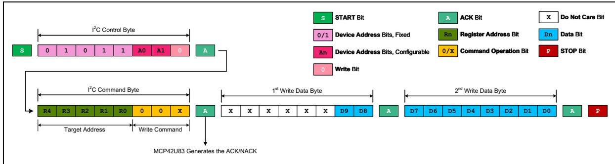
**FIGURE 6-6:** I<sup>2</sup>C Single Write Command Sequence.
