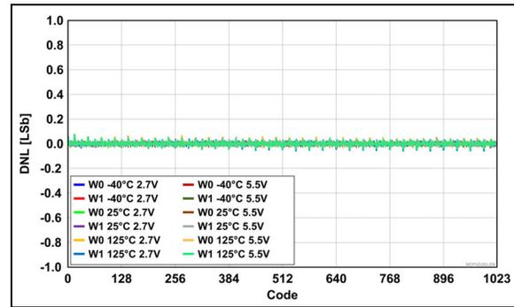
**FIGURE 2-20:** Rheostat Differential Nonlinearity (R-DNL) Error vs. Wiper Position (Code), across  $V_{DD}$  and Temperatures.
