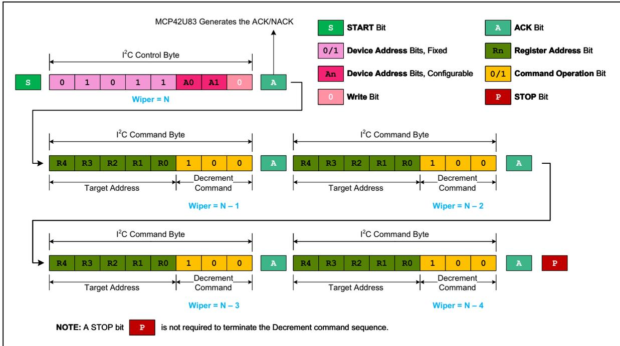
FIGURE 6-12: I<sup>2</sup>C Decrement Wiper Position Command Sequence.
