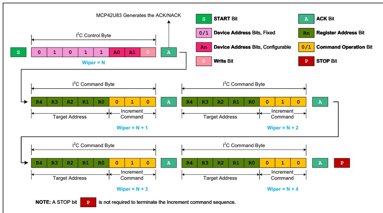
FIGURE 6-11: I<sup>2</sup>C Increment Wiper Position Command Sequence.
