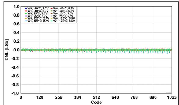
**FIGURE 2-25:** Rheostat Differential Nonlinearity (R-DNL) Error vs. Wiper Position (Code), across  $V_{DD}$  and Temperatures.
