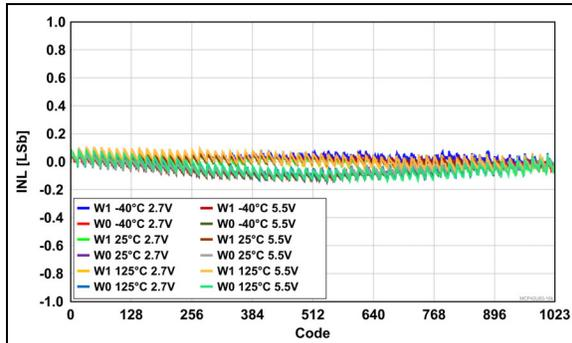
**FIGURE 2-12:** Potentiometer Integral Nonlinearity (P-INL) Error vs. Wiper Position (Code), across  $V_{DD}$  and Temperatures.
