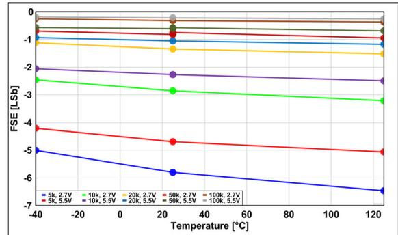
**FIGURE 2-5:** Full Scale Error (FSE) vs. Temperature, across  $V_{DD}$  and  $R_{AB}$ . †
