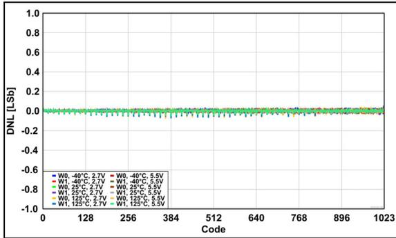
**FIGURE 2-28:** Potentiometer Differential Nonlinearity (P-DNL) Error vs. Wiper Position (Code), across  $V_{DD}$  and Temperatures.
