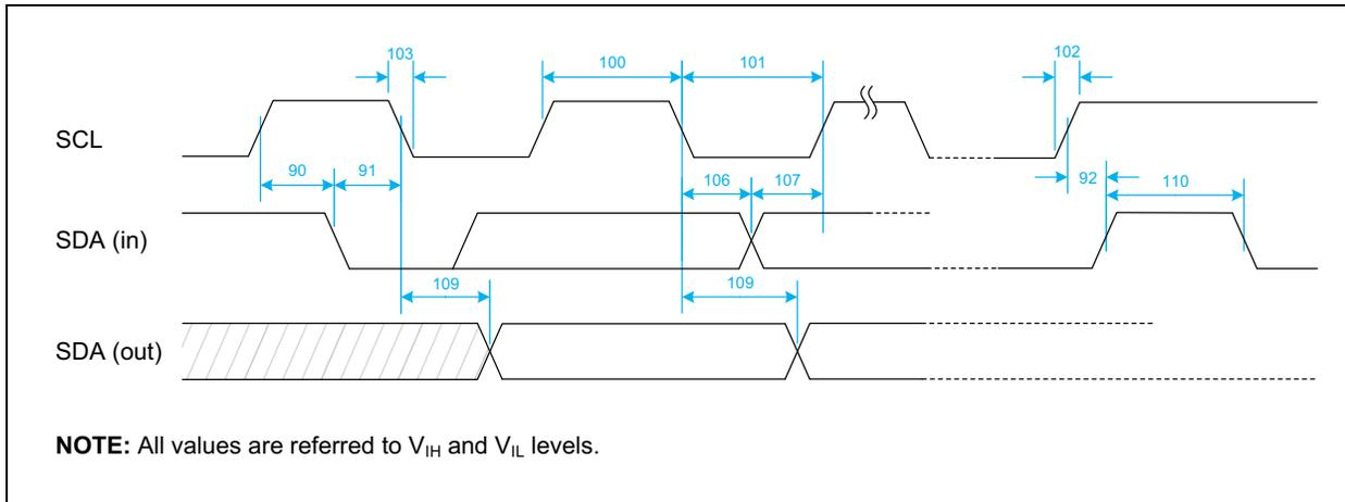
**FIGURE 1-3:** I<sup>2</sup>C Bus Data Timing Waveforms.
