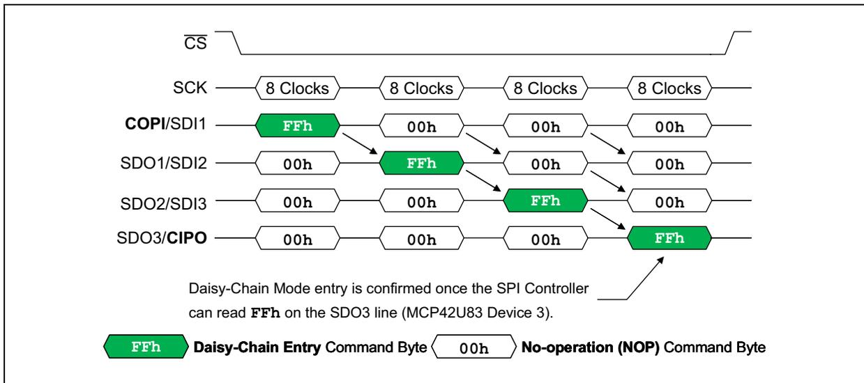
**FIGURE 7-11:** SPI Daisy-Chain Entry Sequence – Example for Three MCP42U83 Devices.
