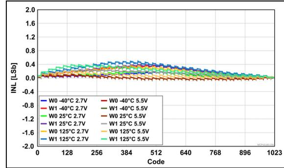
**FIGURE 2-19:** Rheostat Integral Nonlinearity (R-INL) Error vs. Wiper Position (Code), across  $V_{DD}$  and Temperatures.
