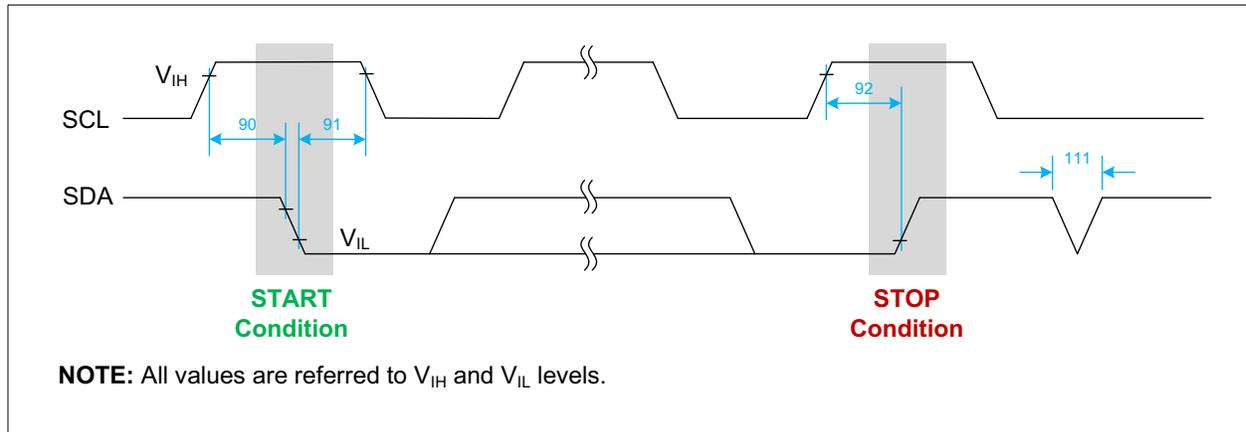
**FIGURE 1-2:** I<sup>2</sup>C Bus Start/Stop Bits Timing Waveforms.
