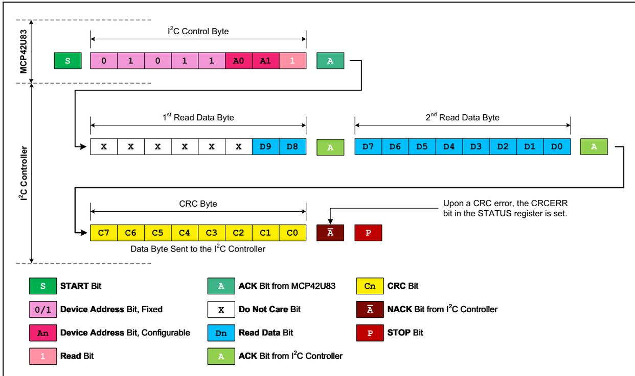
FIGURE 6-17: I<sup>2</sup>C Read Last Accessed Memory Command Sequence with CRC Enabled.
