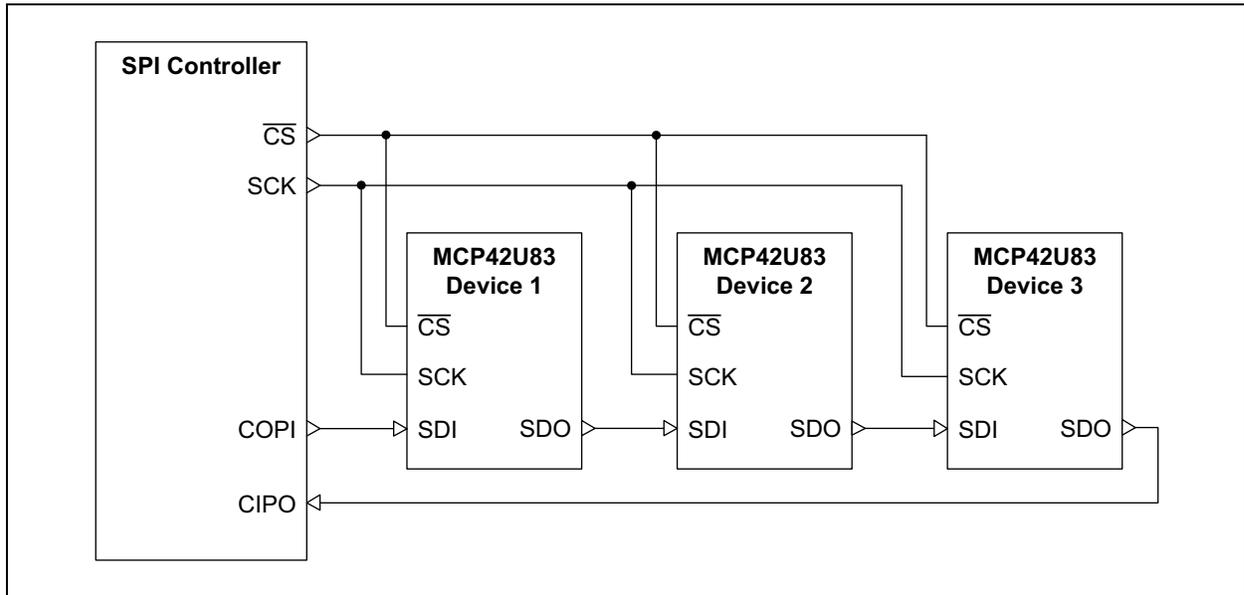
**FIGURE 7-10:** SPI Daisy-Chain Bus Configuration – Connection Example for Three MCP42U83 Devices.
