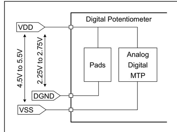
FIGURE 4-2: Dual Voltage Configuration.
