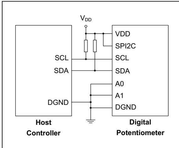
**FIGURE 6-1:** Typical I<sup>2</sup>C Interface Connections.
