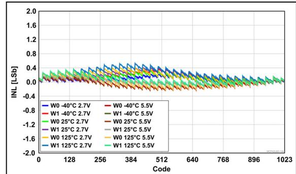
**FIGURE 2-14:** Rheostat Integral Nonlinearity (R-INL) Error vs. Wiper Position (Code), across  $V_{DD}$  and Temperatures.
