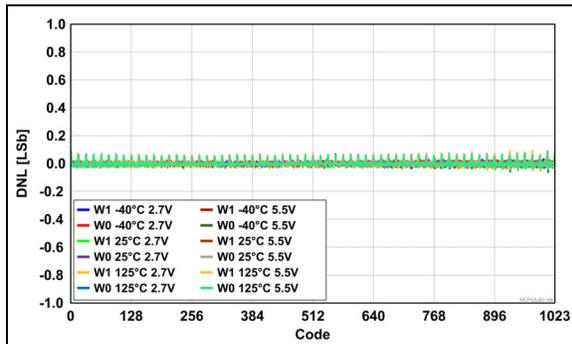
**FIGURE 2-13:** Potentiometer Differential Nonlinearity (P-DNL) Error vs. Wiper Position (Code), across  $V_{DD}$  and Temperatures.
