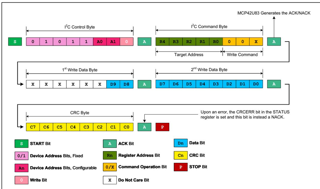
FIGURE 6-13: I<sup>2</sup>C Write Command Sequence with CRC Enabled.
