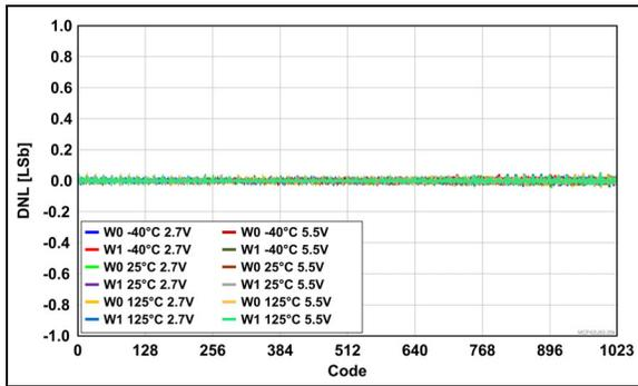
**FIGURE 2-18:** Potentiometer Differential Nonlinearity (P-DNL) Error vs. Wiper Position (Code), across  $V_{DD}$  and Temperatures.
