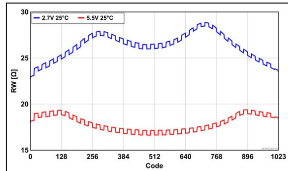
**FIGURE 2-11:** Wiper Resistance ( $R_W$ ) in Rheostat Mode vs. Wiper Position (Code), across  $V_{DD}$  and Temperature.
