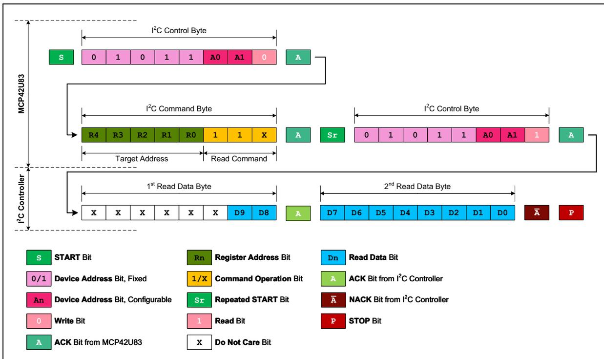
FIGURE 6-8: I<sup>2</sup>C Read Random Address Command Sequence.
