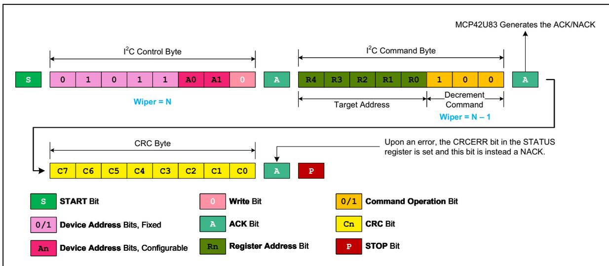
FIGURE 6-15: I<sup>2</sup>C Decrement Command Sequence with CRC Enabled.
