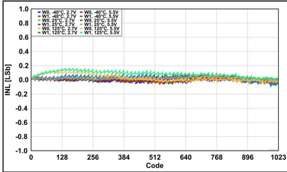
**FIGURE 2-27:** Potentiometer Integral Nonlinearity (P-INL) Error vs. Wiper Position (Code), across  $V_{DD}$  and Temperatures.
