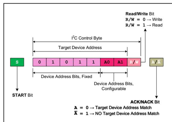
**FIGURE 6-2:** Target Device Address Bits of the I<sup>2</sup>C Control Byte.
