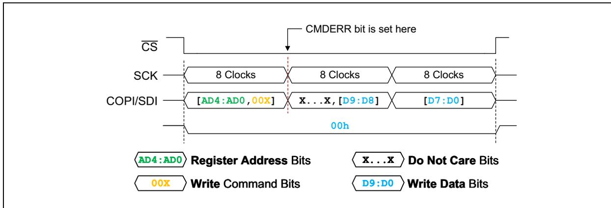
FIGURE 7-7: SPI Write Command – SDI and SDO States.
