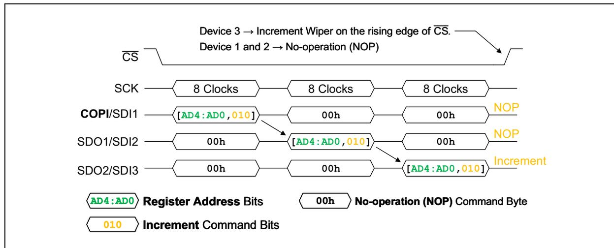
**FIGURE 7-14:** SPI Daisy-Chain Addressable 8-Bit Increment/Decrement Commands Example.
