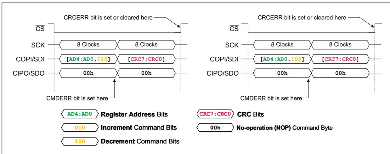
FIGURE 7-18: SPI Increment/Decrement Command Sequence with CRC Enabled.
