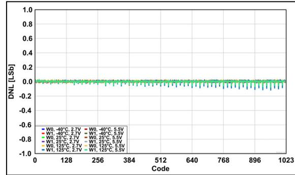
**FIGURE 2-30:** Rheostat Differential Nonlinearity (R-DNL) Error vs. Wiper Position (Code), across  $V_{DD}$  and Temperatures.
