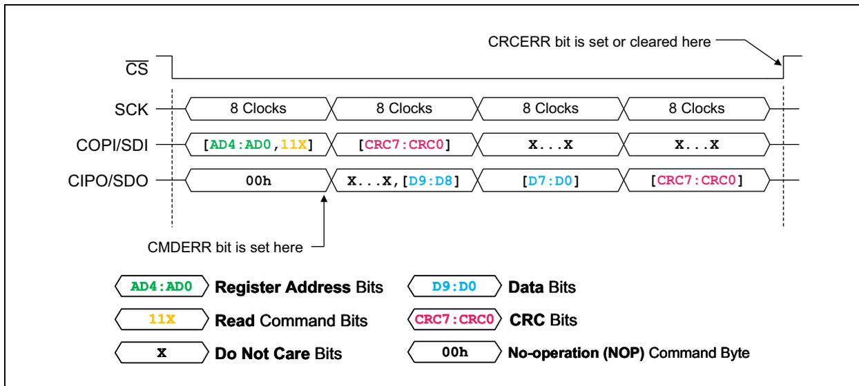
**FIGURE 7-19:** SPI Read Command Sequence with CRC Enabled.
