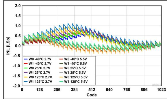
**FIGURE 2-9:** Rheostat Integral Nonlinearity (R-INL) Error vs. Wiper Position (Code), across  $V_{DD}$  and Temperature.
