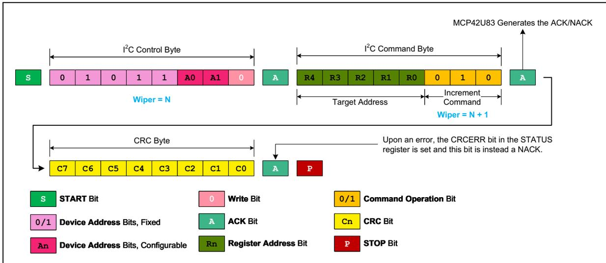
FIGURE 6-14: I<sup>2</sup>C Increment Command Sequence with CRC Enabled.
