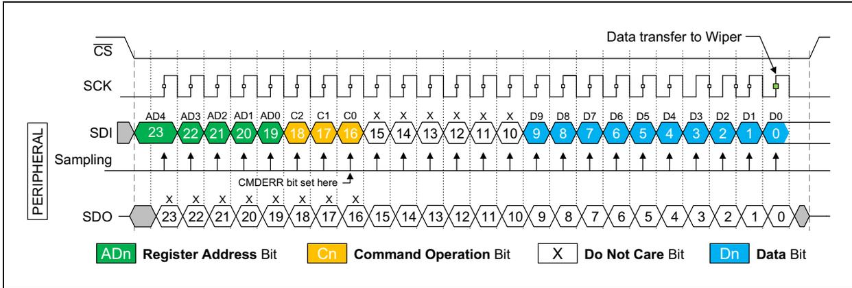
**FIGURE 7-4:** 24-Bit Commands (Write, Read) – SPI Mode (0,0) Waveform.
