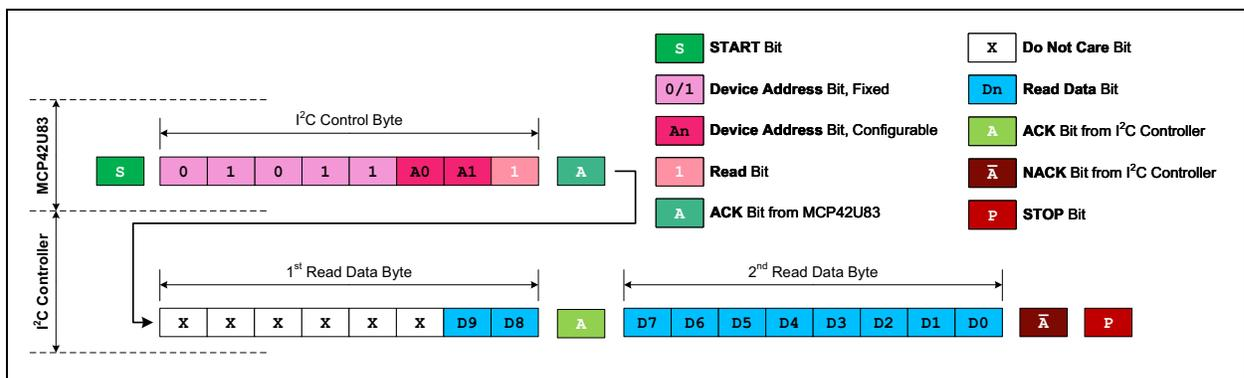
**FIGURE 6-9:** I<sup>2</sup>C Read Last Memory Address Command Sequence.
