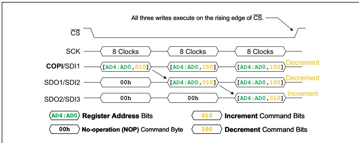
FIGURE 7-12: SPI Daisy-Chain 8-Bit Increment/Decrement Commands Example.
