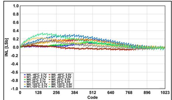
**FIGURE 2-24:** Rheostat Integral Nonlinearity (R-INL) Error vs. Wiper Position (Code), across  $V_{DD}$  and Temperatures.
