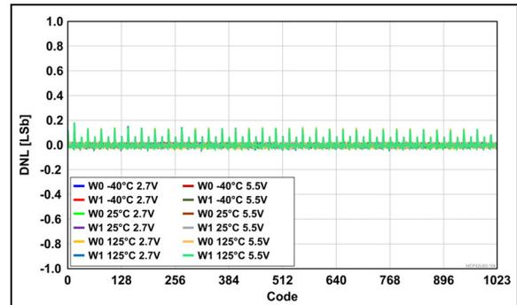
**FIGURE 2-15:** Rheostat Differential Nonlinearity (R-DNL) Error vs. Wiper Position (Code), across  $V_{DD}$  and Temperatures.
