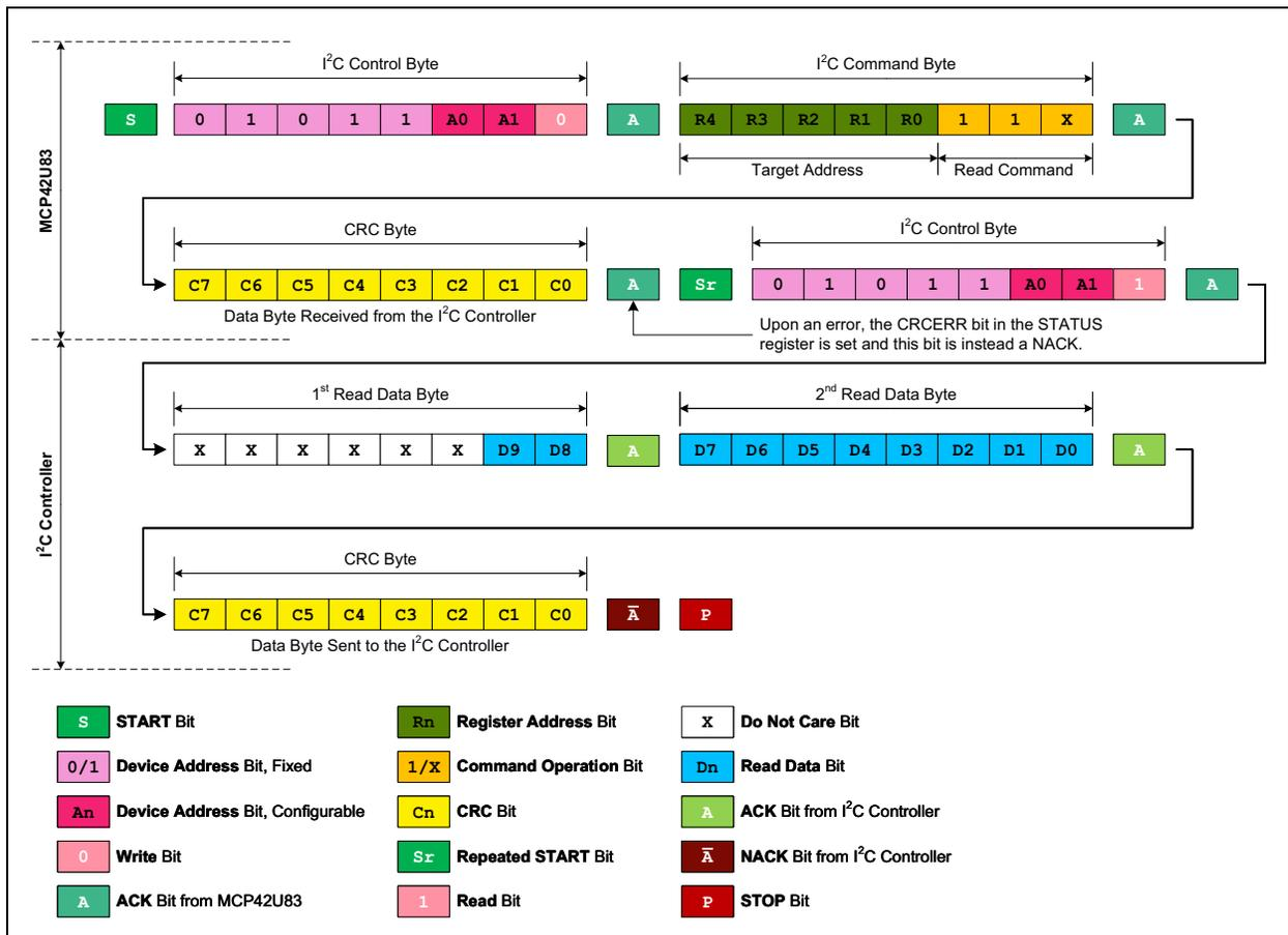
FIGURE 6-16: I<sup>2</sup>C Read Random Address Command Sequence with CRC Enabled.
