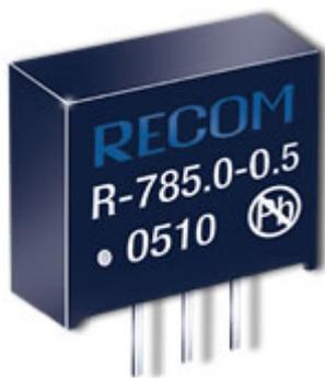
The R-78xx-0.5 offers output voltages from 1.5V to 15VDC at a maximum output current of 0.5A with the full input voltage range of up to 34VDC. The SIP3 package measures only 11.5 x 10 x 8mm (0.45 x 0.4 x 0.3"), yet delivers up to 7.5 Watts of power. The R-78xx-1.0 offers output voltages from 1.8V to 5VDC at a maximum output current of 1A with a reduced input voltage range of 4.75 to 18VDC in the same package.
