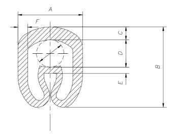
LFHG is a specially designed expandable marker to grip a wide range of cable sizes. The chevron end cut enables locked alignment of a series of legends.
