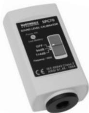
Output sound pressure levels: 94dB and 114dB rel 20 $\mu$ Pa under reference conditions
