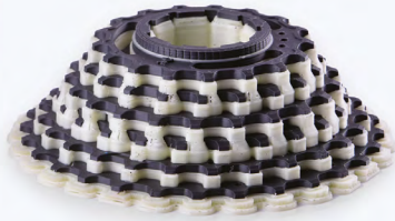
Bicycle cassette model before support material dissolution
