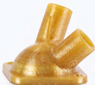
Temperature resistant thermostat housing 3D printed with Z-PEI 1010
