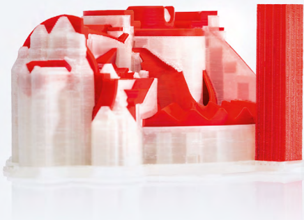
Model of gear mechanism before support material dissolution
