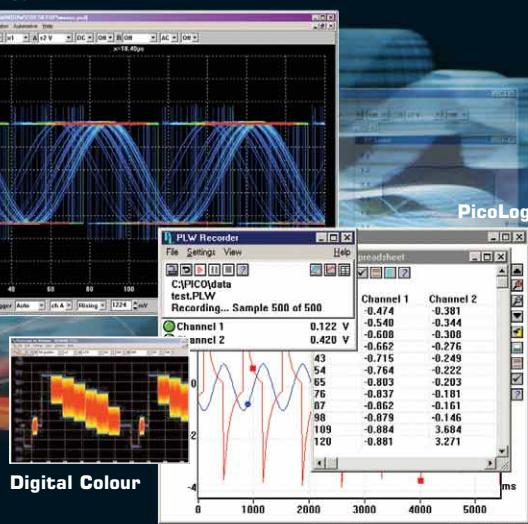
The PicoScope 3000 series PC oscilloscopes incorporate PicoScope software that turns your PC into an oscilloscope and spectrum analyser. PicoLog data acquisition software, also supplied, transforms your PC into a high speed data logger.
