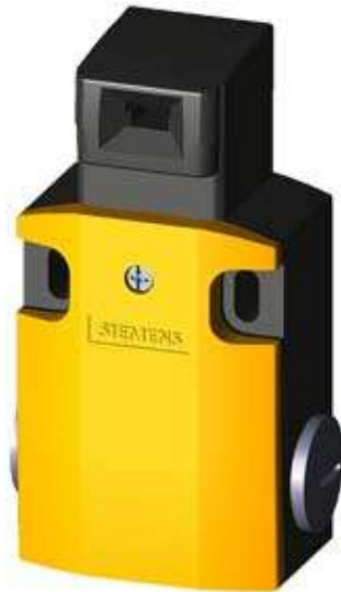
SAFETY POS. SWITCH W. SEPARATE ACTUATOR, METAL HOUSING, 56MM, DEVICE CONNECTION 3X (M20X1.5) SLOW-ACTION CONTACTS 2NC/1NO 5 DIRECTIONS OF APPROACH
