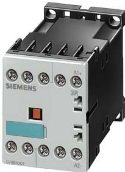
COUPLING RELAY, 4NO, DC 24 V, 0.7...1.25*US, W.DIODE SCREW CONNECTION, SIZE S00
