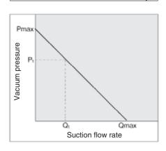
Flow characteristics are expressed in ejector vacuum pressure and suction flow. If suction flow rate changes, a change in vacuum pressure will also be expressed. Normally this relationship is expressed in ejector standard supply pressure.
