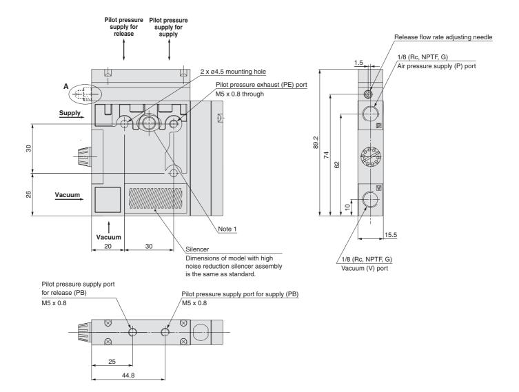
Note 1) This is a hole for using the manifold and single unit bodies in common, and it is not used for the single unit.
