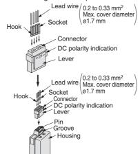
**2. Crimping of lead wires and sockets** Strip 3.2 to 3.7 mm of the lead wire ends, insert each stripped wire into a socket and crimp contact it using special crimping tool. Be careful that the outer insulation of the lead wires does not interfere with the socket contact part.
