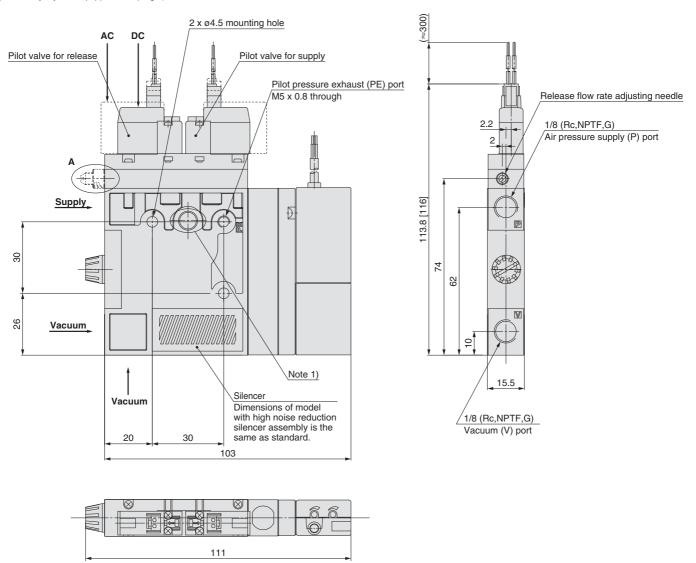
Note 1) This is a hole for using the manifold and single unit bodies in common, and it is not used for the single unit. Note 2) [ ]: AC
