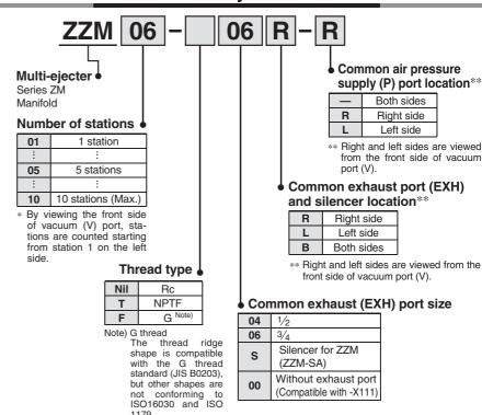
The asterisk (\*) indicates the ejector model no. below the manifold base no. Prefix it to the vacuum ejector part numbers to be mounted. When it is not added, products are shipped separately.
