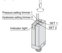
· When using the switch to confirm correct adsorption, the vacuum pressure is set to the minimum value to reliably adsorb. If the value is set below the minimum, the switch will be turned ON even when adsorption has failed or is insufficient. If the pressure is set too high, the switch may not turn ON even though it may adsorb correctly.
