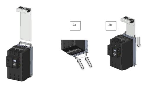
Step 3. When the fan assembly is fully home and the lower plate of the assembly has engaged with the lower mounting screws, re-tighten the mounting screws fully.
