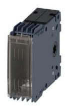
Accessory for 3KF size 1 Fourth pole, switchable for LV HRC fuse Sz. 000 flat terminal on the rear
