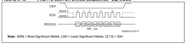
FIGURE 5-20: 4 KBYTE SECTOR-ERASE SEQUENCE (SPI)
