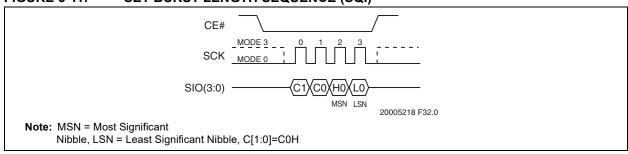
FIGURE 5-12: SET BURST LENGTH SEQUENCE (SPI)
