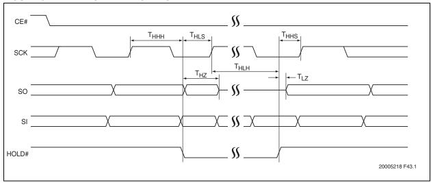
FIGURE 8-2: SERIAL INPUT TIMING DIAGRAM
