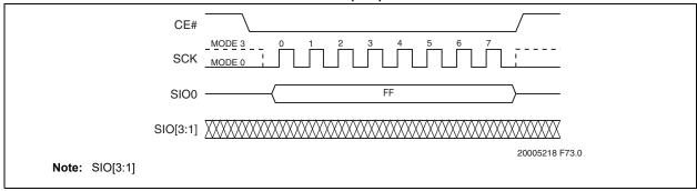
FIGURE 5-5: RESET QUAD I/O SEQUENCE (SQI)
