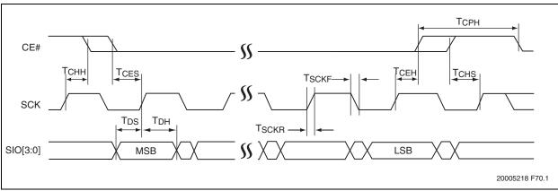
FIGURE 8-3: SERIAL OUTPUT TIMING DIAGRAM
