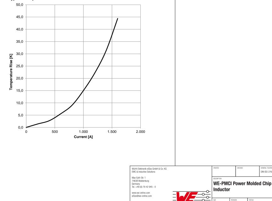
**Typical Temperature Rise vs. Current Characteristics:**
