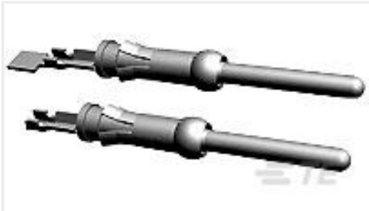
TE Part #66361-3 III+ PIN,18-14,15AU/FL,LP
