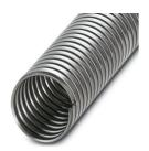
Protective hose, material: Stainless steel 1.4301/AISI 304, degree of protection: IP40, color: silver, inside diameter: 40 mm, Total length: 10 m
