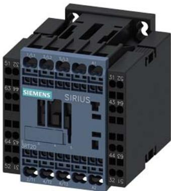
power contactor, AC-3e/AC-3, 12 A, 5.5 kW / 400 V, 3-pole, 110 V DC, with integrated diode, auxiliary contacts: 2 NO + 3 NC, spring-loaded terminal, size: S00, 3RH2921-2DA11 (1 NO + 1 NC), mounted left and right
