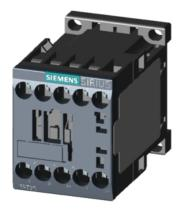
power contactor, AC-3, 16 A, 7.5 kW / 400 V, 4-pole, 110 V AC, 50/60 Hz, main contacts: 2 NO + 2 NC, screw terminal, size: S00
