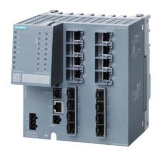
SCALANCE XM408-8C; managed modular IE switch; 8x 10/100/1000 Mbit/s RJ45; 8x 100/1000 Mbit/s SFP; contains 8 combo ports; in total 8 ports can be used; expandable to 24 ports electrical or optical; assembly: DIN rail/S7 mounting rail, PROFINET IO device; redundancy functions; office features (RSTP, VLAN, IGMP,..); C-plug in scope of delivery; Layer 3 with key plug available
