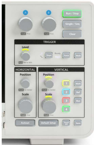
Simplified and intuitive front panel with color coded LEDs
