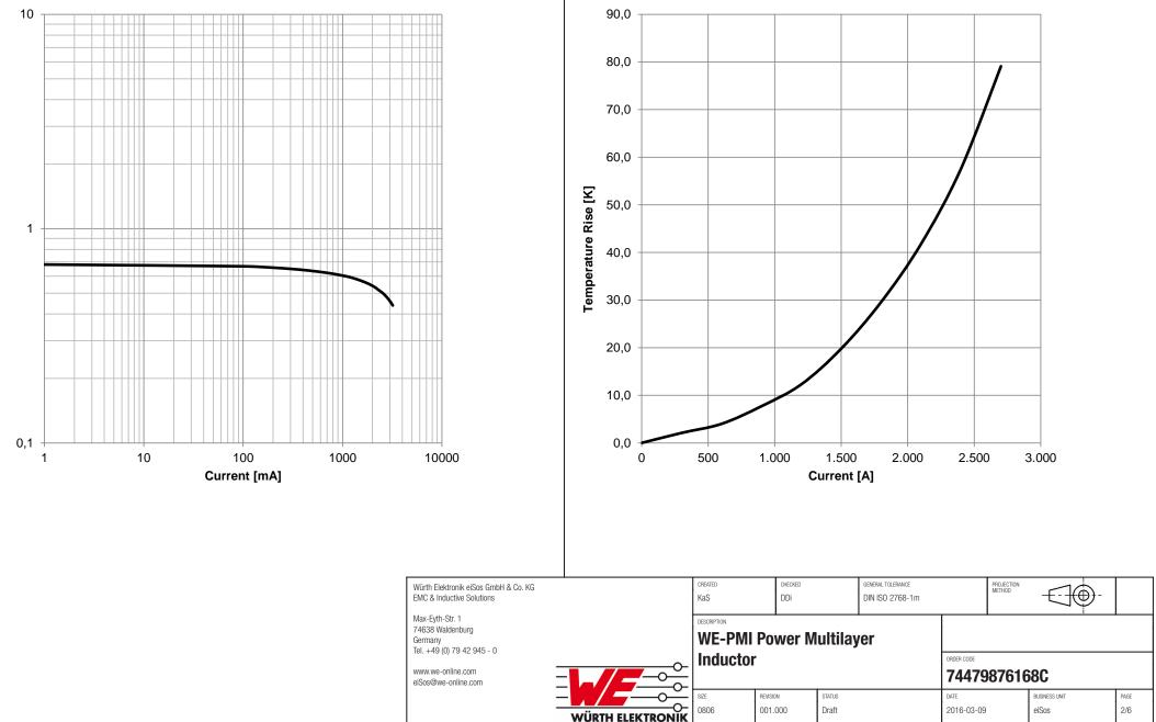
**Typical Temperature Rise vs. Current Characteristics:**
