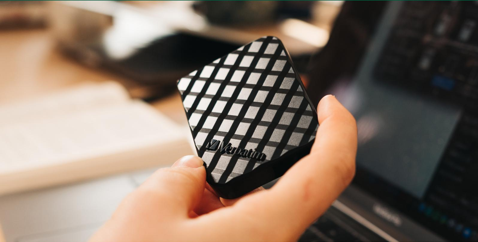
SSDs are generally more durable and reliable. There are no moving parts to damage and no drive motor to break. So, in addition to being used for internal computer storage, this reliability makes SSDs great for portable, external drives, which may be subject to more rigorous use and handling. Apart from these benefits, SSDs have a range of other advantages. We've listed a quick summary for you below.
