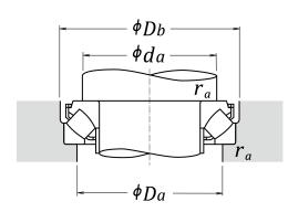
Abutment diameter spacer ring
