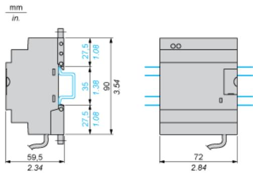
Screw Mounting (Retractable Lugs)
