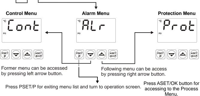
**NOTE :** If Process Output Selection **Cout** is **SSr**, after Alarm-1 parameters, Alarm-2 parameters can be observed.
