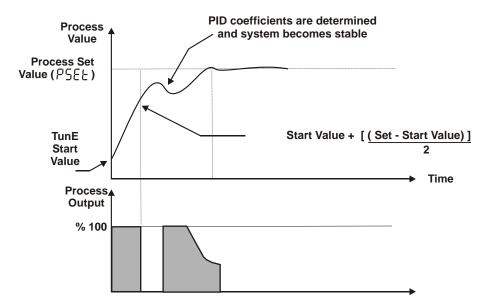
If cooling function and PID control form is selected for the system;
