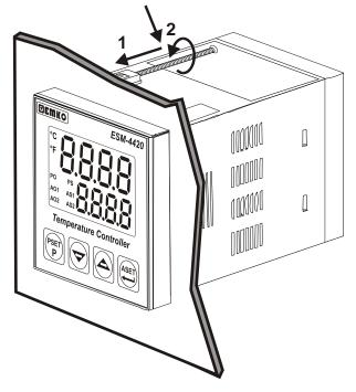
The unit is designed for panel mounting.
