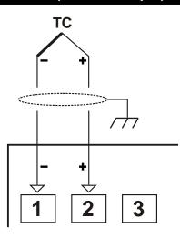
Connect the wires with the polarity as shown in the figure left.
