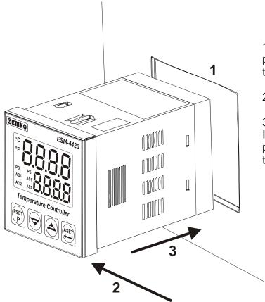
1-Before mounting the device in your panel, make sure that the cut-out is of the right size.
