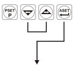
Press ASET/OK button for saving the changes and accessing to the following parameter.
