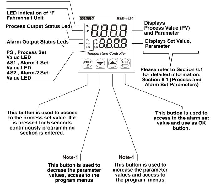
Note-1: If increment or decrement button is pressed for 5 seconds continuously, increment and decrement number become 10, if increment or decrement button is pressed for 10 seconds continuously, increment and decrement number become 100.
