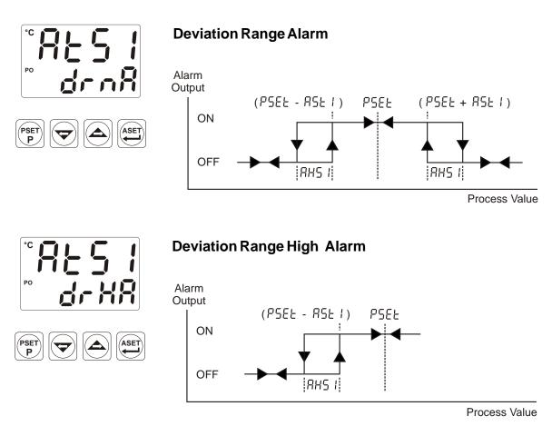
**Note :** If the one of  $dH_1R$ ,  $dL_0R$ ,  $db_0R$ ,  $dc_0R$  and dcHR these alarm types are selected, alarm set value can be decreased to zero with the decrement button even though alarm set low limit is negative value.
