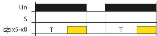
When the supply voltage "Un" is applied, the time delay "T" starts. The output contact(s) " " will close after the delay has elapsed. If the supply voltage "Un" is disconnected, the output contact(s) " " are opened and the function is reset. Control input "S" is not used in this function.
