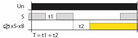
When the supply voltage "Un" is applied while the control input "S" is closed, the time delay "T" doesn't start. The delay only starts when the control input "S" is open. The output contact(s) " " will close after the delay has elapsed. If the supply voltage "Un" is disconnected, the output contact(s) " " are opened and the function
