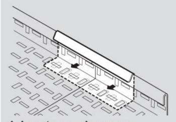
1. Locate coupler across underside of tray joint
