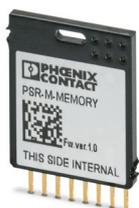
Optional memory block for the PSRmodular system for easy storage and backup of configuration data. When using the PSR-M-B3 base module, use the memory card from item revision 1105142-1.
