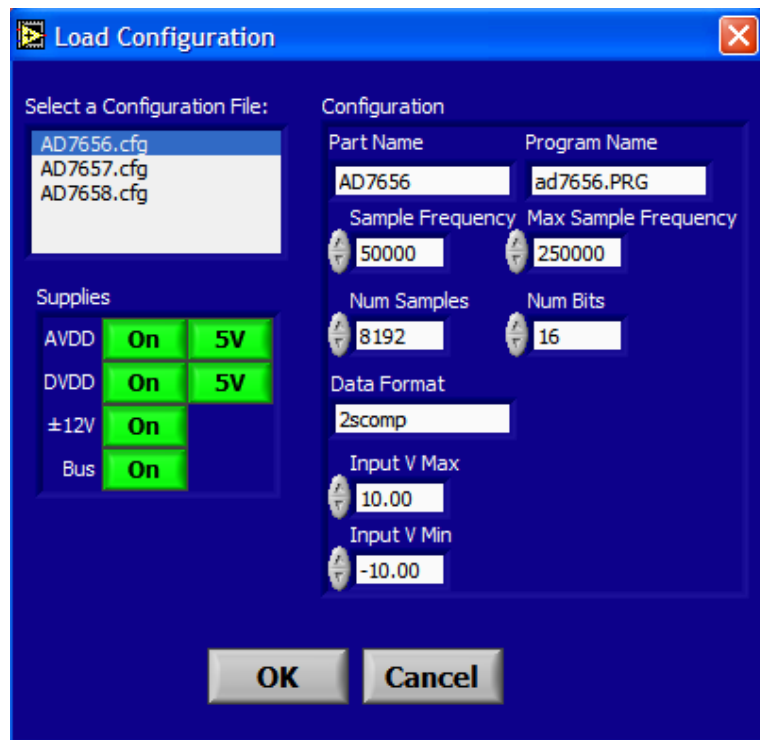
Figure 4. AD7656 Evaluation Software, Load Configuration Window
