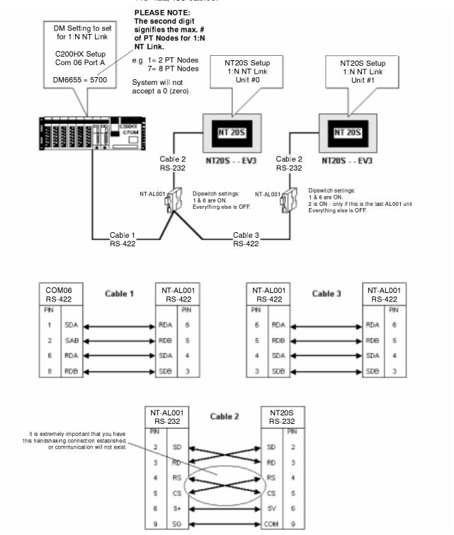
**Reference:** When connecting the C200HX/HG/HE and an RS-232C/RS-422 converter unit, use a converter unit whose lot number is 15Y5 or later. Converter units of lot numbers previous to 15Y5 cannot be connected.
