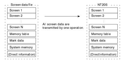
When the screen data is transmitted from the support tool to the NT20S, the screen data already existing in the NT20S will be erased.
