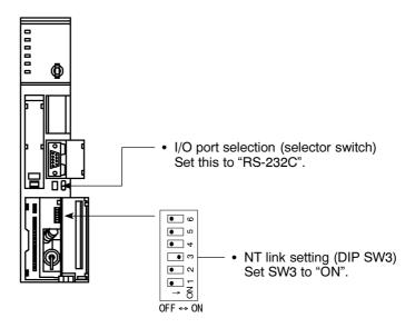
When using CVM1/CV series, always set CPU execution processing (execution control 2) in the PC system settings to simultaneous processing.
