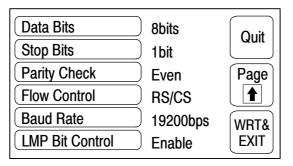
Each time the "LMP Bit Control" touch switch is pressed, the setting option "Enable" alternates with "Disable".
