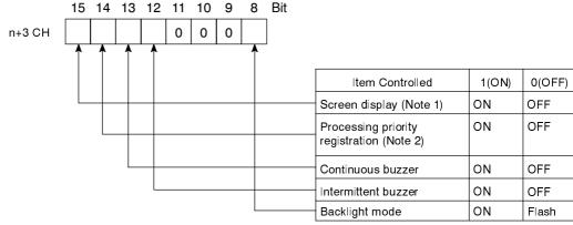
Note 1:When "ON" is set for screen display, the backlight is on; when "OFF" is set for screen display, the backlight is off.
