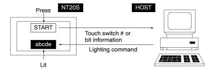
Bit touch switch method (bit input permitted setting)
