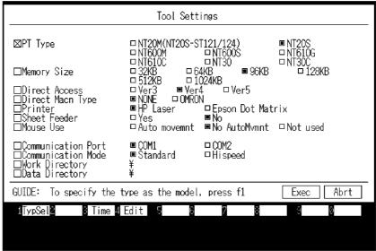
To create the NT20S screen data, make settings in the "Tool Settings" screen as follows.
