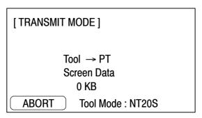
**6.** When the screen data transmission is completed, the support tool will display the following screen.
