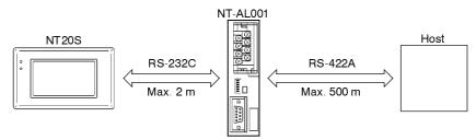
**Reference:** When connecting the C200HX/HG/HE and an RS-232C/RS-422A converter unit, use a converter unit whose lot number is 15Y5 or later. Converter units of lot numbers previous to 15Y5 cannot be connected.
