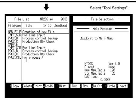
Select a file used for storing the screen data for the NT20S in the "File List" screen.
