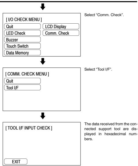
When the check is finished, press the Exit touch switch. The NT20S will enter the I/O CHECK MENU.
