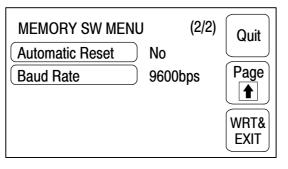
Each time the "Automatic Reset" touch switch is pressed, the setting option "Yes" alternates with "No".
