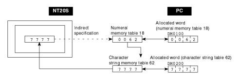
In indirect specification, the contents (numerical value) of the specified numeral memory table are regarded as a memory table number and the contents of the table with this number are displayed.
