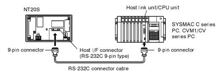
**Note:** The connector cable wiring for the C series CPU unit (C□□H) is different from that for the other PCs. For details, refer to Appendix G Method for Making the Cable for Connection to the Host (page 256).
