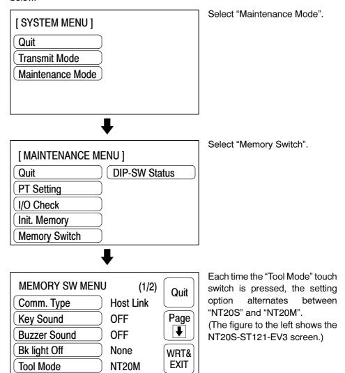
To quit after setting the selected item, press the WRT & EXIT touch switch. To quit without setting, press the Quit touch switch. The NT20S will enter the RUN mode.
