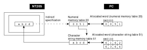
This specification method is a little complex, but it allows the display to be changed more easily according to the circumstances. In the example above, if 1 were added to the contents of memory table 20 to give 52, the contents of memory table 52 would be displayed instead.
