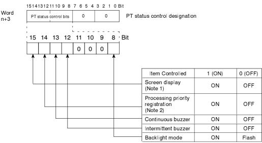
Note 1: The backlighting is on when the screen display bit is set to ON and off when the screen display bit is set to OFF.
