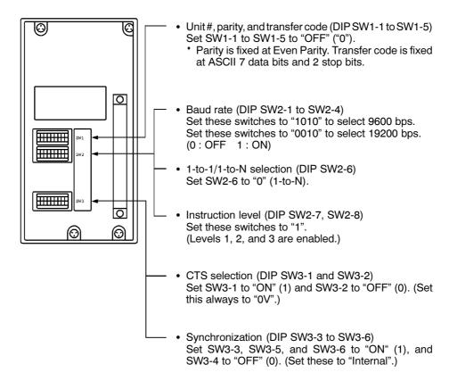
CVM1/CV series backplate mounted type: CV500-LK201
