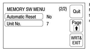
Repeatedly pressing the "Unit No." touch switch cycles through the numbers that can be set.
