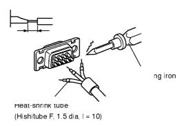
(4) Push the heat-shrink tube over the soldered joint and heat the tube to shrink it in place.
