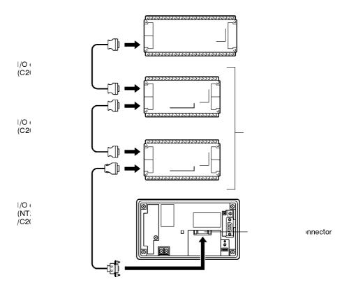
**Note:** When connecting a C□□H, always install a noise filter.
