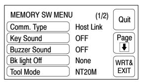
Repeatedly pressing the "BK light Off" touch switch cycles through the setting options "10 min", 1 hour, and None, in that order.
