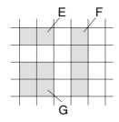
If switches E and F are turned ON at the same time, switch G is also set ON.
