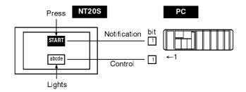
In order to notify the status of a touch switch to the PC, the touch switch must be allocated to a specified PC bit so that it can be managed. Designate the area and bit number.
