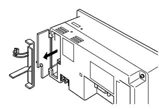
3. Re-install the backlight and connect its connector to the NT20S. Close the cover and tighten the screw with a flat-head screwdriver.
