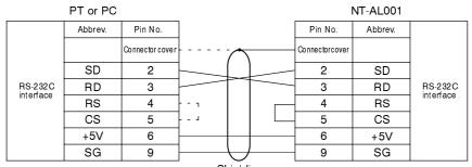
The pin numbers are the numbers at the NT20S. Shielding - - - Only connected at PC For the pin numbers at the PC, refer to the manual for the PC used.
