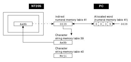
**Reference:** This method is convenient when switching the display at the same location, for example when monitoring a series of words, or when using unique codes to specify individual character strings, etc.
