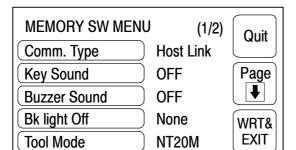
Each time the "Key Sound" touch switch is pressed, the setting option "ON" alternates with "OFF".
