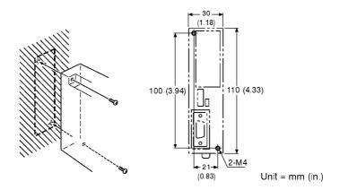
**Note:** In order to ensure a strong installation, the wall of the operation panel must be at least 2 mm thick.
