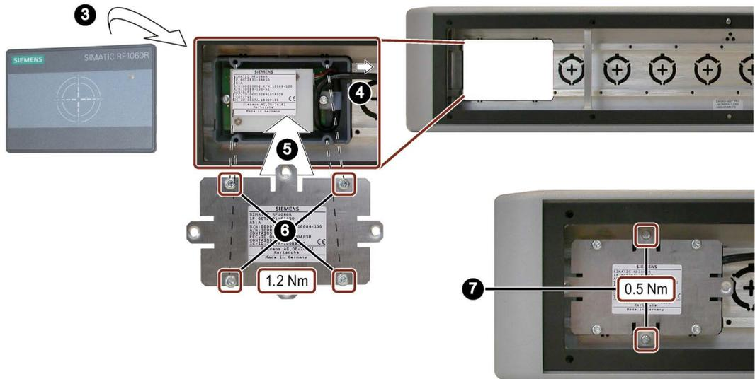
4. Guide the USB cable of the reader through one of the cutouts to the outside of the reader housing.
