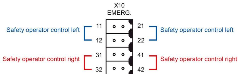
Internal wiring in the Extension Unit using the example of an emergency stop button:
