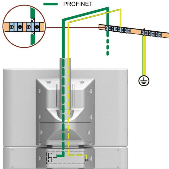
The rail for functional grounding should be installed close to the Extension Unit or the device. Route the functional grounding cable and the data cables in parallel and with minimum clearance in between.
