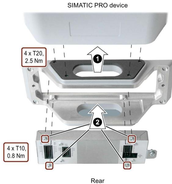
1. Fasten the connection compartment onto the PRO device as shown below with a torque of 2.5 Nm using the 4 screws and the angled T20 screwdriver included in the product package.
