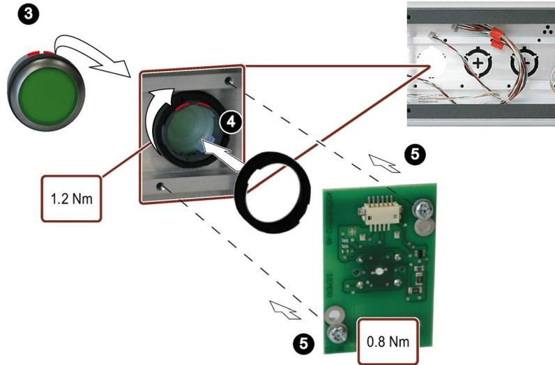
4. Fasten the operator control from the inside with the supplied nut, torque = 1.2 Nm.
