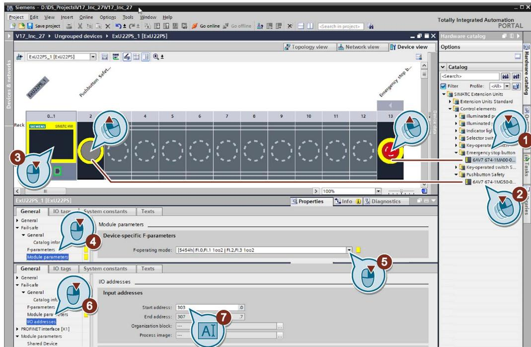
1. In the device view of the Extension Unit 22" PROFSafe, drag the emergency stop button from the catalog tree to "Rack" position 13.
