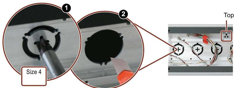
2. Cut out the foil at the required mounting position with a sharp knife. Notice! Only cut within the cutout. To ensure a tight fit, the foil cutout can be smaller but not larger than the cutout for the operator control.
