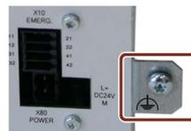
3. Connect the cable for functional grounding to the corresponding connector of the control cabinet from which the Extension Unit is supplied with power.
