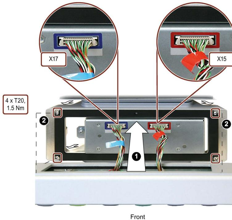
1. Attach the front of the Extension Unit to the connection compartment as shown and connect the 30-pin connector of the cable harness to the interfaces X15 and X17 of the communication module. The cable harnesses of the connectors are marked with colored adhesive tape as follows:
