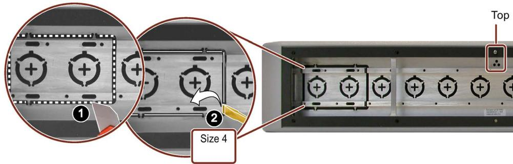
2. Insert a screwdriver size 4 as shown in a gap of the screw bar and carefully lift out the metal plate. If the metal plate does not release completely, use the screwdriver and insert it into a different gap of the screw bar.
