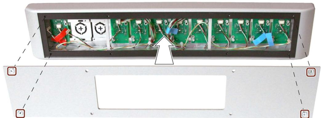
Tighten the 4 marked screws with a torque of 1.5 Nm.
