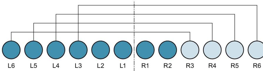
Connected slots must only be occupied by one standard operator control, either left (L) or right (R).
