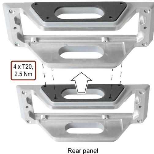
Stand mounting: Fasten the connection compartment to the mechanical interface of the stand with 4 T20 screws and a torque of 2.5 Nm.
