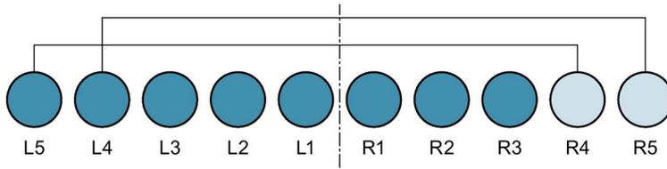
Connected slots must only be occupied by one standard operator control, either left (L) or right (R).
