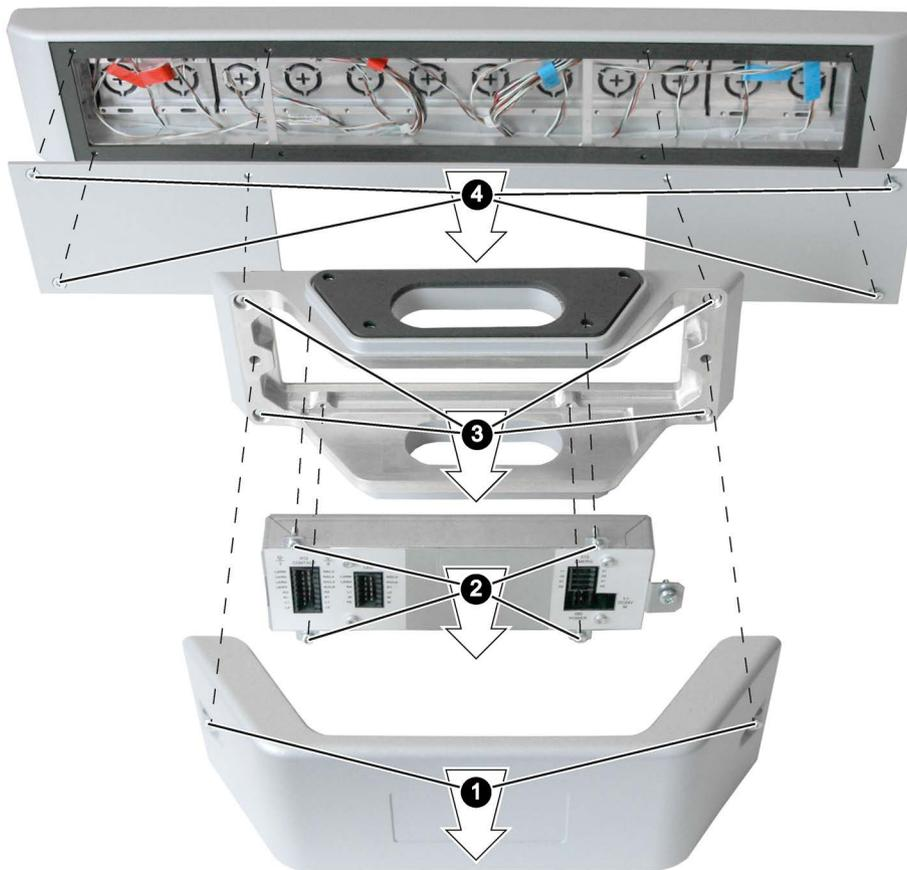
1. Loosen the 2 screws of the terminal compartment cover with a T20 screwdriver and remove the terminal compartment cover.
