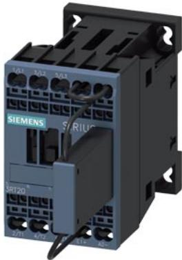
traction contactor, AC-3e/AC-3, 12 A, 5.5 kW / 400 V, 3-pole, 72 V DC, 0.7-1.25\* Uc, with integrated suppressor diode, auxiliary contacts: 1 NC, spring-loaded terminal, frame size: S00, with plugged on series resistor
