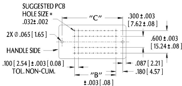
SOCKET FOOTPRINT (top view - component side)
