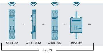
Wireless Protocol Operating frequency range: 2400-2483.5 MHz Maximum output power: 10 dBm EIRP
