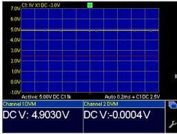
■ Here is the result for the driver with a faulty open circuit output. The output is pulled to 5V by the active pull-up in the CircuitMaster. and the results is a horizontal line at 5V and a 5V (approx) DVM reading.
