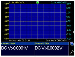
Let's explain. The CircuitMaster uses *Active* mode to impose an active load on the probe, using a programmable voltage source in conjunction with a selectable series resistance. With an open circuit, the input voltage follows the active load voltage (1V nominal, actually 0.9842V measured by the DVM), but with a short circuit the input is still 0V as in the right hand picture.
