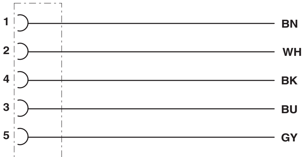
Contact assignment of the M12 socket
