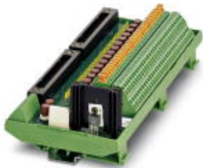
VARIOFACE input module, 32 channels for Yokogawa input modules ADV151, ADV161.
