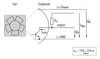
All voltages measured to ground. External load resistor  ${\rm R}_{\rm A}$  from  ${\rm U}_{\rm A}$  to  ${\rm U}_{\rm BA}$  required.
