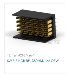
120 Position High Speed Backplane Connector, 12 Row, 10 Column, PCB Mount Receptacle, Vertical, Unshrouded, 1.9 mm [.075 in] Centerline, Z-PACK TinMan
