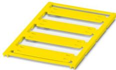
Cable marker, Sheet, yellow, unlabeled, can be labeled with: BLUEMARK E.CARD, BLUEMARK ID COLOR, BLUEMARK ID, BLUEMARK CLED, PLOTMARK, CMS-P1-PLOTTER, mounting type: Assembly with cable ties, cable diameter: > 7 mm, Number of individual labels: 4, text field height: 15 mm, text field width: 44 mm
