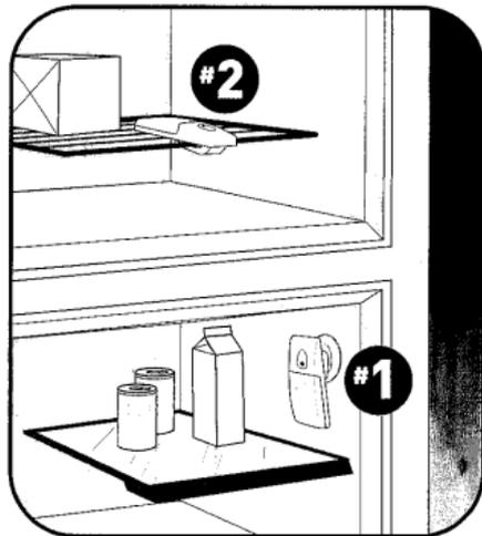
The main unit may be mounted directly to the refrigerator surface utilizing the magnetic back of the unit. The main unit may also be placed on a table or other flat surface using the integrated fold-out stand on the back of the unit.
