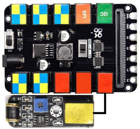
It is compatible with the Micro:bit board and the TS2179 Micro:bit expansion board.
