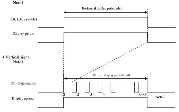
Note1: This diagram indicates virtual signal for set up to timing. Note2: See "**4.9.3 Input signal timing chart**" for numeration of pulse.
