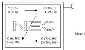
Figure1. Normal scan (DPS: Low or Open)
