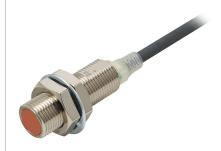
Proximity Sensor, Cylinder type (with screw), Sensing distance: 3 mm, Shielded, DC 2-wire, NO, Pre-wired model, Polarity, Polyurethane cable (oil resistant and reinforced), 2 m
